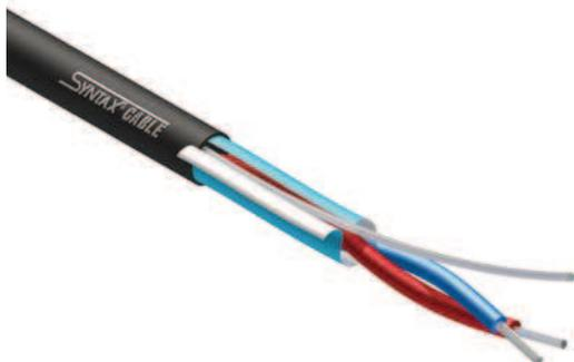
Thanks to its small external diameter, this cable represents the best solution for the internal wiring of racks and audio equipment installations. It is made up of a twisted pair of tinned OFC conductors and tinned drain wire. The XLPE conductor insulation is particularly resistant to high temperatures, so as to avoid warping or shrinkage when soldering. The aluminium/polyester foil shield provides 100% protection from external noises and the tinned drain wire allows faster installation.
