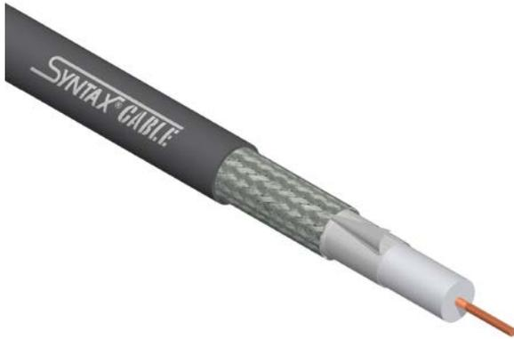
The 7XVD59RHD coaxial video cable meets all the requirements of the Broadcast installations for HDTV and SDI high-definition video in spite of its reduced diameter. The inner conductor insulation is made of a special foam plastic polymer which guarantees a very low capacitance value. This is key to maintaining low damping values on high frequency interconnections even in case of lengthy connections.
