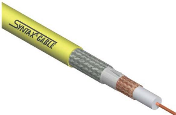
This SYNTAX® halogen free video coax cable 75 Ω is designed for HDTV high performance applications. The inner conductor insulator is made of a special foam plastic polymer to guarantee a very low value of capacitance also for great length connections.
